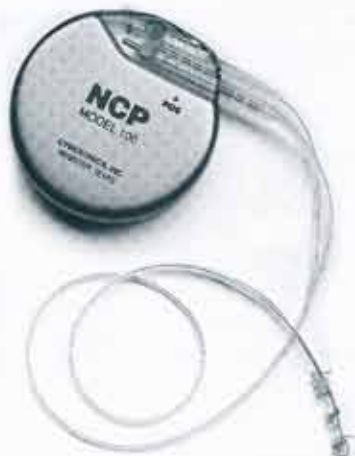
The electrical generator and wire leads
